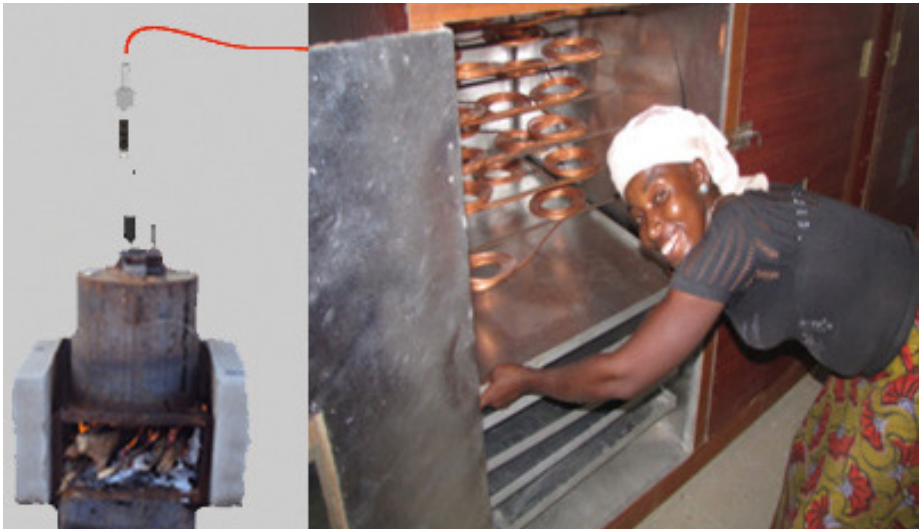
Moving from traditional sun-drying to labour-saving and innovative steam drying technology
